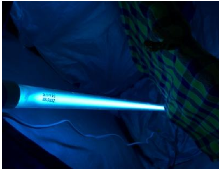
Figure 8 Disinfection process on napkin by ZW30S19W UV lamp for twenty minutes (1200 seconds)
