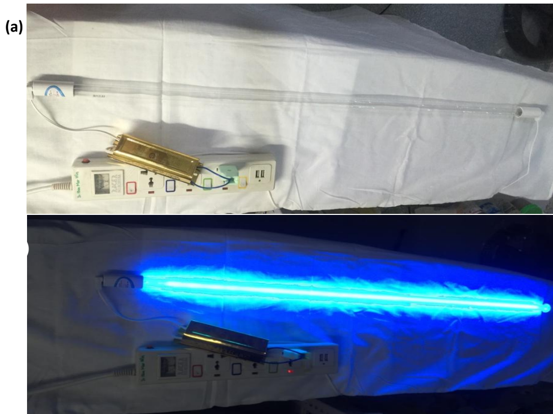
Figure 2 Photograph of the ZW30S19W UV lamp (a) testing circuit connection (b) emitting UV radiation in 253.7 nm wavelength and 107 \mu\text{W}/\text{cm}^2 intensity
